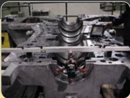
A. Measuring the diaphragms and bearing journals in a turbine.
