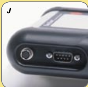
Countersunk connectors, well protected against external damage.
