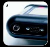
Countersunk connectors, well protected against external damage.
