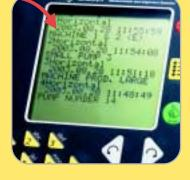
**PRINT** Quickly print all measurement data locally. This is useful, for example, if you don't want to connect the display unit to a PC.
