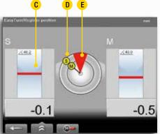
**2.** Take the measurement values in three positions with as little as 20° between.
